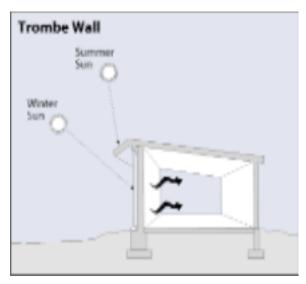
8" wall at noon will heat the inside of the building at 8 PM. The air circulates naturally to heat a room. Fans can be used to heat multiple rooms.
