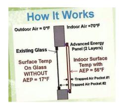
The graphic at left illustrates and quantifies the benefit: while the outside temperature is 17 degrees, the surface of the panel remains at 56 degrees. The photo at right is an Advanced Energy Panel installed in a HOW.
